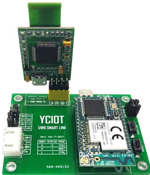
Figure 1.1.2 Mini3 + UWB Smart Link
