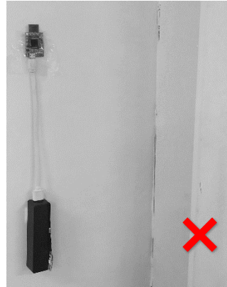
Glue the module to the wall
