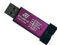
Figure 6.2.1 PHYSICAL IMAGE OF THE STLINK DOWNLOADER
