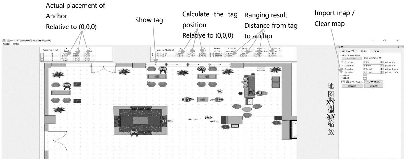
Figure 6.2.1 RTLS host computer interface
