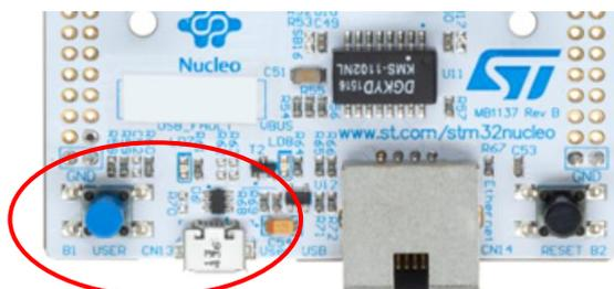
**Figure 5.2.1 STM32 USB virtual serial port**
