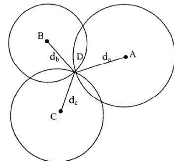
**6.5.1 The Theoretical Basis of Trilateral Measurement Method Based on UWB Ranging**
