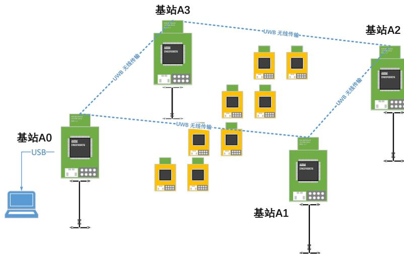
**Figure 4.2.3 Schematic diagram of positioning 4 anchors + multi-tag hardware platform**
