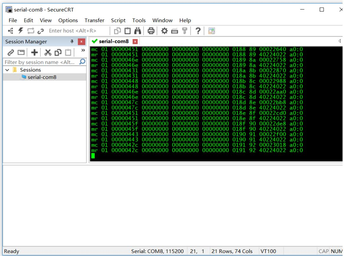
**Figure 5.2.2 Screenshot of STM32 USB virtual serial port data content**
