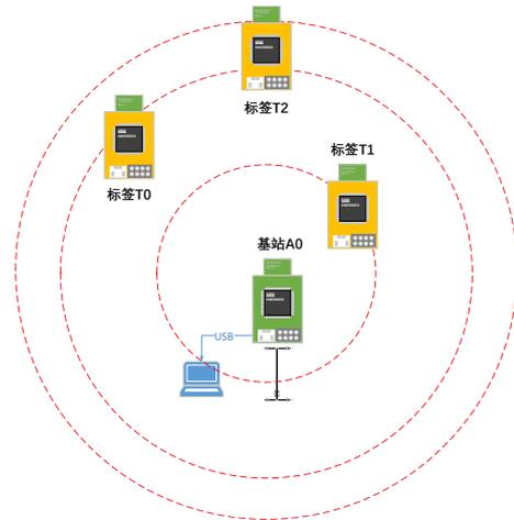
**Figure 4.3 Schematic diagram of over-range alarm 1 anchor + 3 tags hardware platform**
