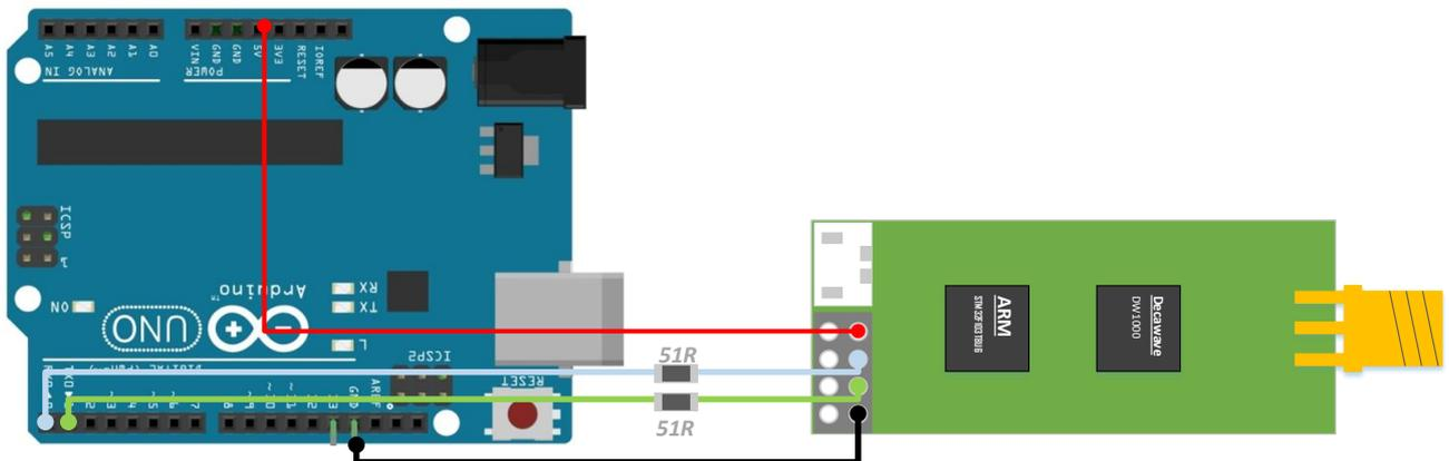
Figure 6.3.1.2 UWB Mini3s module and SCM (Arduino) connection
