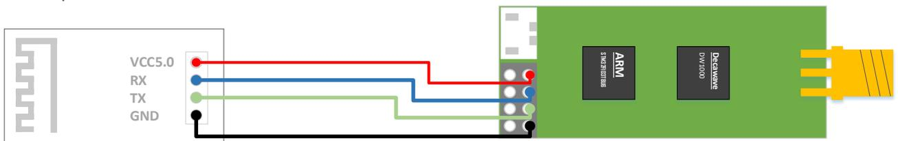
Figure 6.3.1.2 UWB Mini3s module and Bluetooth module connection
