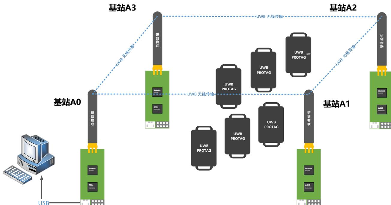
Figure 4.2.3 The schematic diagram of locating 4 stations + multi tag hardware platform
