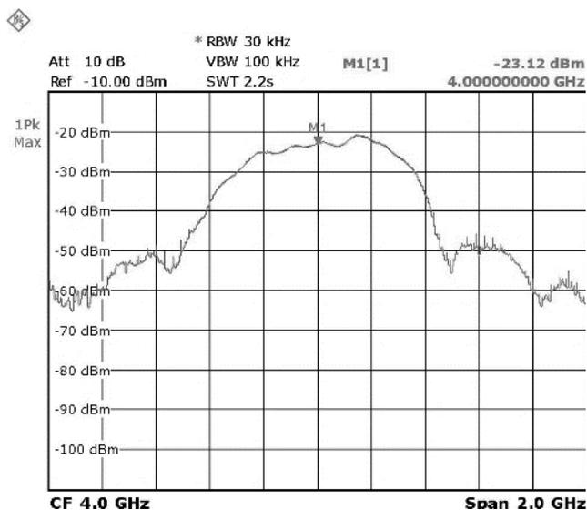
Figure 2.4 ProTag2s Emission power test
