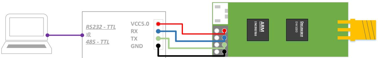
Figure 6.3.1.1 UWB Mini3s module and TTL-RS232 module or TTL-485 module connection
