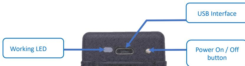
Figure 2.5 UWB ProTag2s Hardware Interface Definition
